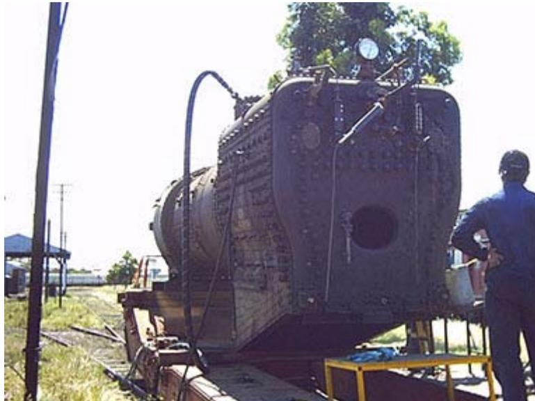
Doing a boiler test on A<sup>2</sup>986 in 2004
